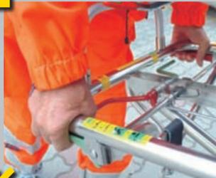
With the left hand grip now the handle on the left side of the stretcher and unlock the rear legs.
