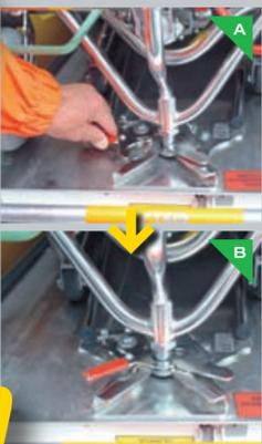
Rotate the stretcher-lock handle towards you, bringing it from position A to position B.
