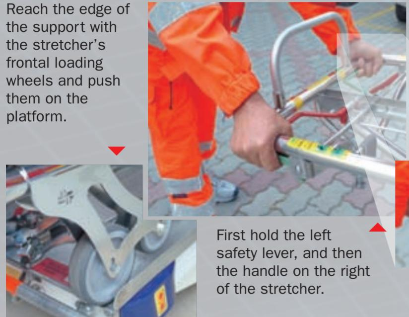
Immediately after push the stretcher on the support, keeping the rear legs on the floor.
