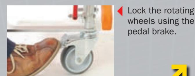
Lock the rotating wheels using the pedal brake.
