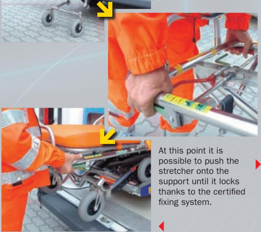
With the left hand grip now the handle on the left side of the stretcher and unlock the rear legs.
