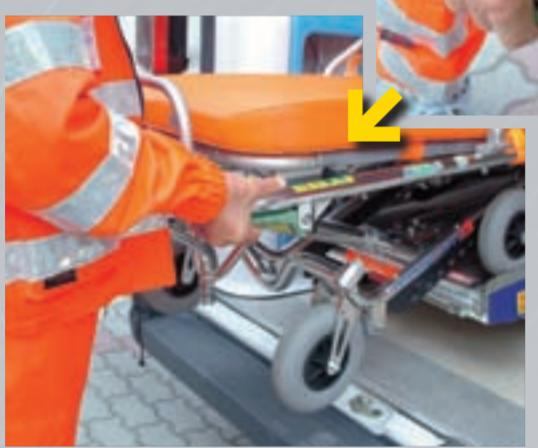
At this point it is possible to push the stretcher onto the support until it locks thanks to the certified fixing system.
