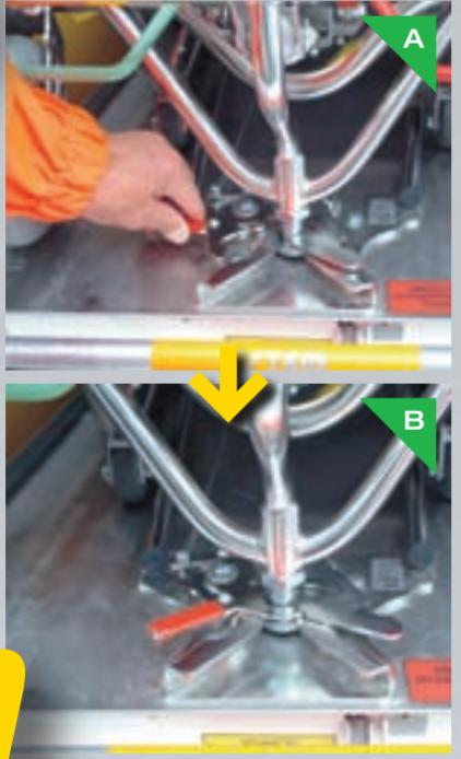
Rotate the stretcher-lock handle towards you, bringing it from position A to position B.
