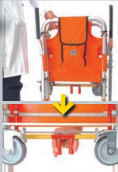
Move to the side of the chair. Hold the chair with one hand and with the other one grip the central levers. Squeeze and unlock the safety-catch.
