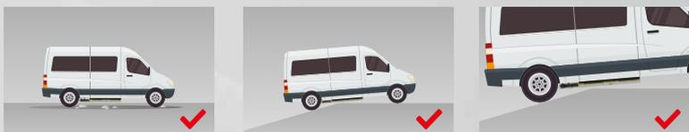
**Opening the step mechanically is dependent on the opening of the side door of the vehicle.**
